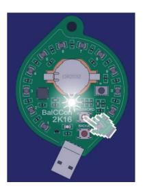
**SWITCH OFF:** The unit will automatically switch OFF after all of the TV codes have been transmitted. You can also switch the badge OFF at any moment by pressing the lower button. Rotating LED pattern in a CCW direction signifies that the unit is OFF.
