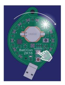
**SWITCH OFF:** The unit is automatically swithced OFF after it is disconnected from the USB port. You can also switch it OFF at any moment by pressing the lower button. A Rotating LED pattern in CCW direction signifies that the unit is OFF.
