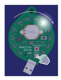
**SWITCH OFF:** Press and release the lower button again. Rotating LED pattern in CCW direction signifies that the unit is OFF.
